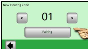
The control unit waits for a receiver in the "RF ini" mode
