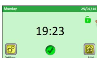
On the new screen, press the "Lock" button to lock the display.
