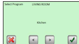
Select the program of another zone with (<) and (>), then press the Valid button: program is automatically renamed with the same name as the current zone. The program created in this way can be subsequently altered without changing the previous program.
