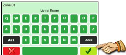
Key "Aa1" is used to switch to the different keyboards (letters, uppercase, numbers, and special characters)
