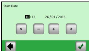
Set the selected parameter (inversely backlit) using the (+) or (-) buttons; move the cursor to the next parameter using the (<|>) buttons at the edges of the screen and validate when OK
