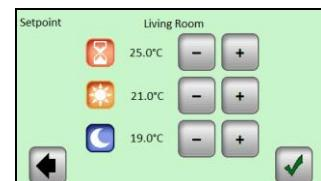
Set the required temperature values with the help of (+) or (-). Confirm or cancel the change by pressing the relevant button in the bottom part of the display.
