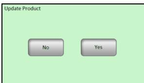
If a valid file is on the SD card when pressing OK, the update process starts. If the file is not valid the message "Abort: SD file not OK", if it is the case then check the file on the SD card and retry process. If the same message appears then the file must be corrupted and you need to download the file again.
