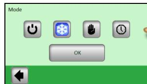
Press the required operating mode, which will highlight it, and confirm your selection by pressing the (OK) button.
